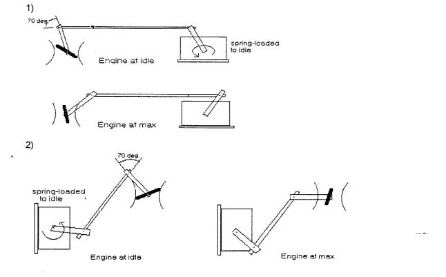
The needed **travel** of the carburetor determines how far out on the Actuator arm the rod is to be attached. In most cases, the carb should be moved from closed to about 10 degrees from full open as the actuator is moved from min to max. Then alter the length of the rod slightly (Perhaps .030"), so that the actuator is just off its internal stop, and is pulling the butterfly against its stop. This insures that the carb can fully close to idle on load dumps, minimizing overspeeds.
